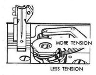
TENSION ON THREAD SHOULD BE AS LIGHT AS POSSIBLE WHILE STILL SUFFICIENT TO SET STITCH
