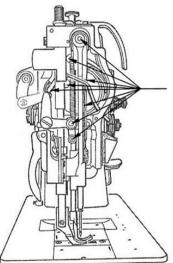
THESE LUBRICATION POINTS MUST BE OILED IN ADDITION TO ALL THE OTHER POINTS BEFORE THE MACHINE IS PLACED IN OPERATION FOR THE FIRST TIME
