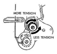
REGULATE NEEDLE THREAD TENSION ONLY WHEN PRESSER FOOT IS DOWN
