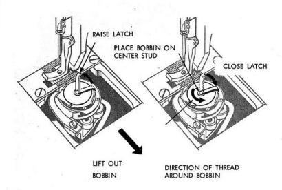
BOBBIN CASE CAP REMOVAL AND REPLACEMENT 211 G 665-01, 211 G 665-02, 211 G 666-01 AND 211 G 666-02 MACHINES
